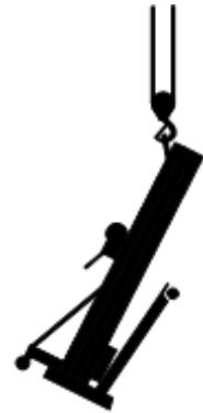
Always place the lifting hook through the lifting eye so that it points away from the machine.
