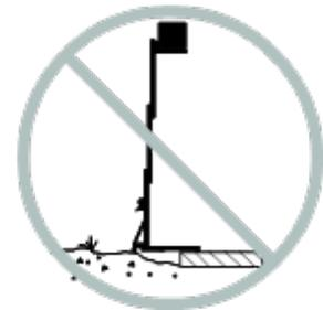
Prior to use, check the work area for drop-offs, holes, bumps, debris, unstable or slippery surfaces or other possible hazardous conditions.
